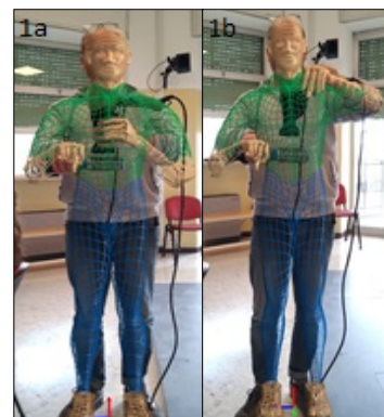
Figure 6: 1a and 1b: images show the frontal view reconstruction made with 3DSSPP software of the posture adopted by the worker in the drying task with holder (1a) and without holder (1b)
