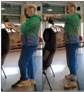
Figure 7: 2a and 2b: images show the side view reconstruction made with 3DSSPP software of the posture adopted by the worker in the drying task with holder (2a) and without holder (2b)
